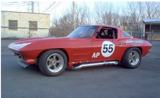
Correct spoiler and wheel openings for C2
